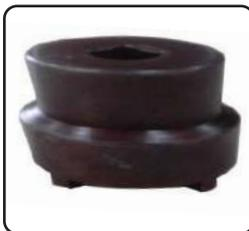
Steering Bearing Adjusting Nut Socket
