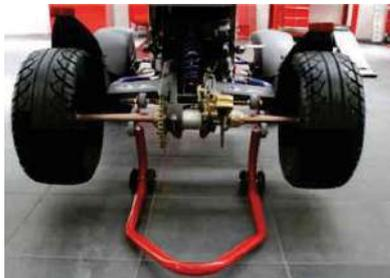
Stand developed and produced for the rear lift of Quads, made by a single steel pipe of 35mm diameter and 2mm of wall thickness. The polyhester powder painting ensures a long lasting and prevent by scratches. Equipped with 4 nylon wheels with overall diameters of 90mm, and with roller supports for an easy and comfortable fitting on the rear wheel axle.
